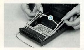
1. Remove the spreader: Use two hands and lift both steel loops (A) together. They are held by springs. The spreader will come out of the camera.
